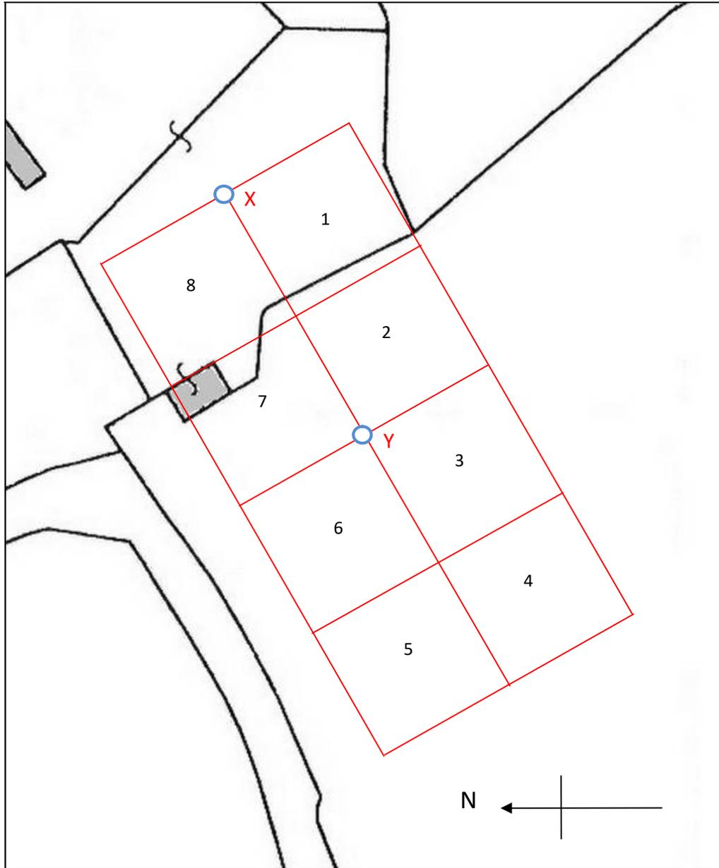
**Figure 3. Survey Area 'A' Grid Layout and Baseline**
